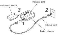
2 Plug the AC plug cord into the power outlet.
