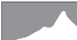
When the image is underexposed, the part to the left is cut off (dark portions) and when the image is overexposed, the part to the right is cut off (bright portions).
