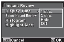
**3** Use the four-way controller (▲▼) to select [Zoom Instant Review], [Histogram] or [Highlight Alert], and use the four-way controller (◀▶) to switch between  (On) and  (Off).
