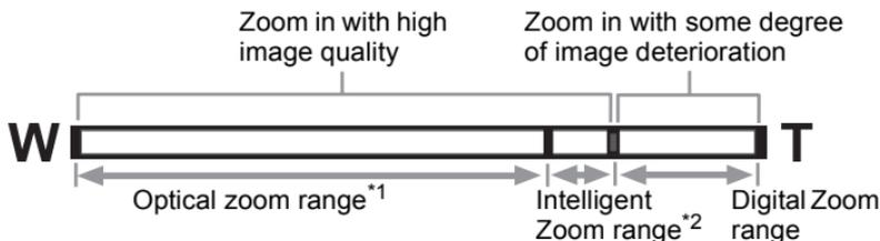
\*1 You can zoom in to a maximum of 4.0x optically (6.0 mm - 24.0 mm (Approx. 28 mm - 112 mm in 35 mm equivalent focal length)).
