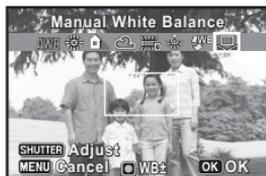
**2** Under the light you wish to measure the white balance of, fully display a white sheet of paper on the display, or select a white area as the subject.
