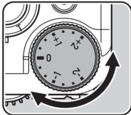
The compensation value is temporarily displayed when adjusted.
