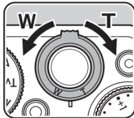
If you continue turning the lever to the right (**T**), the camera automatically switches from optical zoom to Intelligent Zoom and stops at the point it switches to Digital Zoom.
