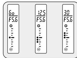
**6** When the shutter release button is depressed halfway down, the shutter speed and aperture value will be displayed in the viewfinder and on the LCD panel.
