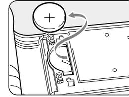
② Reinstall the battery chamber cover, and tighten the battery chamber fixing screw.
