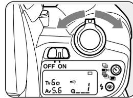
**4** Move the select switch to change the aperture while holding the exposure compensation button.
