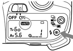
The flash mode will be displayed on the LCD panel as shown below.
