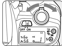
**4** When the shutter release button is depressed halfway down, the shutter speed and aperture value will be displayed in the viewfinder and on the LCD panel.
