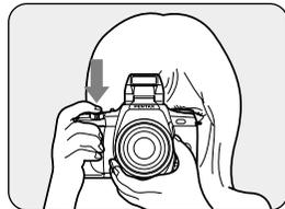
**4** After using the flash, retract the built-in flash by pressing it down into the camera body.
