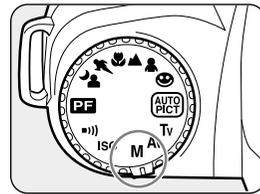
**3** Move the select switch to change the shutter speed.
